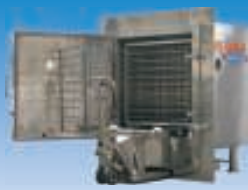
Vacuum tray dryer with extractable shelves
