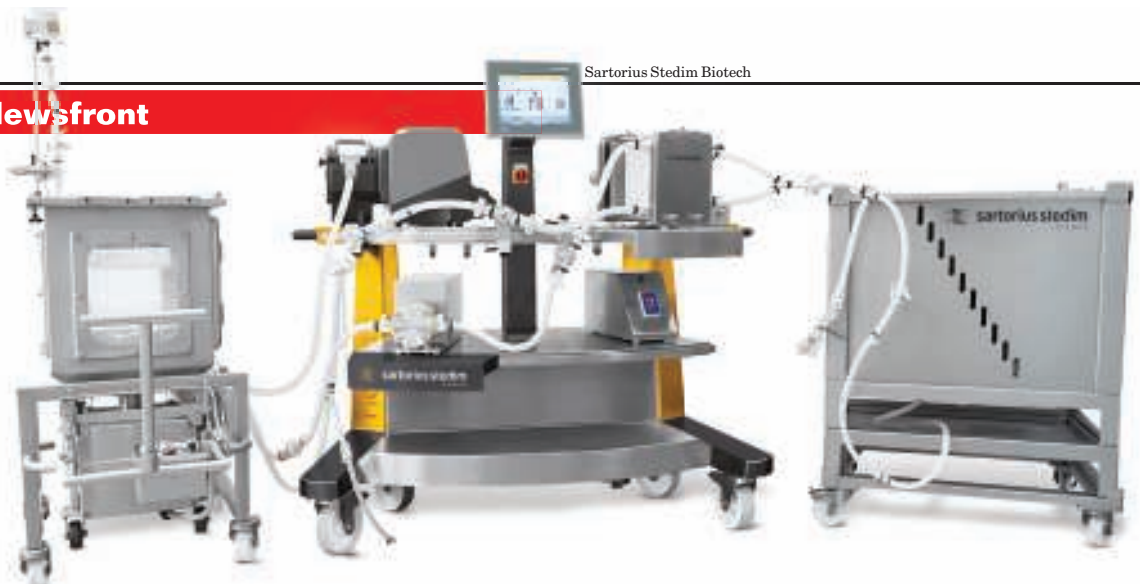
FIGURE 3. FlexAct is a new system that enables custom-configurable single-use solutions for entire biomanufacturing steps
