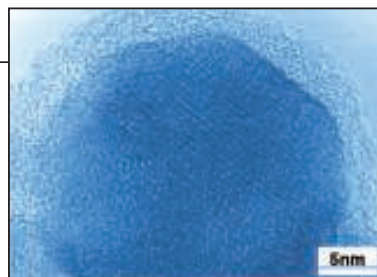
FIGURE 2. Pulsed-plasma techniques, like the one Aeonclad Coatings used to make this epoxy nanocomposite, allow better control of surface chemistry and avoid surface ablation
